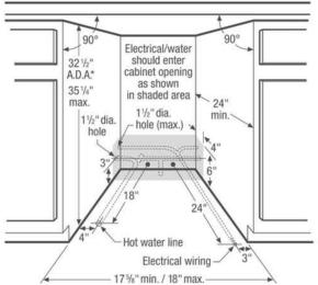
\*A.D.A. installation,  $(32\,1\!/2)$  beneath 34"- high countertop may be accomplished by adjusting toekick and leveling legs.
