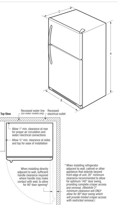
When properly installed, this model is A.D.A.-qualified based on the United States Access Board's A.D.A./A.B.A. Accessibility Guidelines and the Department of Justice's 2010 A.D.A. Standards for Accessible Design. "For use on adequately wired 120V, dedicated circuit having 2-wire service with a separate ground wire. Appliance must be grounded for safe operation.
