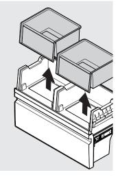
2. Carefully handle the slide-out shelf to prevent making contact with the cabinet liner during removal and installation.
