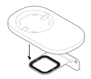
Route the speaker's power cord through the Shelf opening. (You'll wrap the cord around the bottom of the Shelf after it's assembled.)
