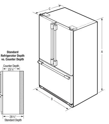
Recessed Recessed **Top View** electrical outlet water line 7 Allow 1" min. clearance at rear for proper air circulation and 24" water/electrical connections 25" Cabinet Countertop 28<sup>7</sup>/<sub>8</sub>" Side Panels, <sup>1</sup>/<sub>2</sub>" min. width
