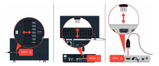
First disconnect and reconnect the power cables and HDMI cables on the back of your TV or the One Connect Box, then unplug the power cord and plug it back into the wall outlet.
