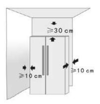
The refrigerator must be placed on hard, flat ground; if cushioning is needed, stable, hard, nonflammable cushion blocks shall be used.
