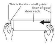
Disassembly: Hold both sides of the door rack with both hands. Push it from the side without the guide and push it inward as seen in the diagram. Push until the edge of the door rack is separated from the grove of the liner.
