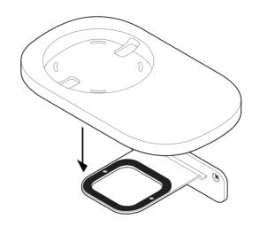
Route the speaker's power cord through the Shelf opening. (You'II wrap the cord around the bottom of the Shelf after it's assembled.)
