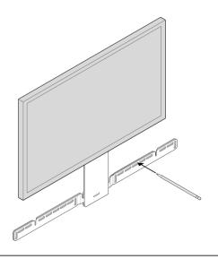
If you're using the included wall anchors, use a 5/16" drill bit to drill the pilot holes and then insert the wall anchors. Don't use the anchors if you're drilling into wood or plastic.
