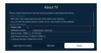
Select > Settings > Support > About TV and check the model code and software version.
