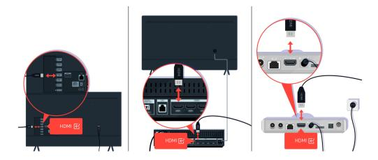
Check the antenna and HDMI cable connections.
