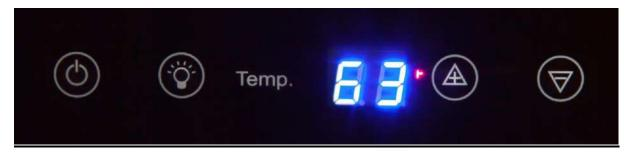
**ON/OFF:** To turn on or off the unit, press this button for 5 seconds.
